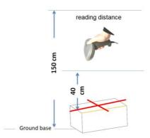
Keep vertical to the upper surface of the carton when measuring, and the best pitch (forward/backward) reading angle and best tilt (leftward/rightward) reading angle is  $\pm 10^{\circ}$  from the ground.
