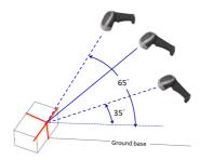
The best skew (leftward/rightward) reading angle is ±7°.
