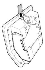
**2.2.2** Insert a Flash USB Drive into any of the available USB ports in the Data I/O compartment or in the side compartment
